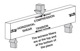
fibers over each other horizontally. This action is similar to the way the ends of playing cards slide over each other when a deck is sharply bent. The internal force that resists this action is the horizontal shear value of the wood. The shearing stress is maximum at the center of the depth of the piece.
