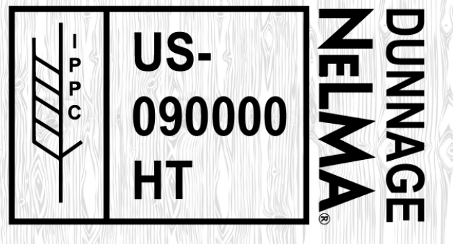
fig. F: A clean impression of a compliant IPPC Dunnage stamp. Note that all information is present and legible.
